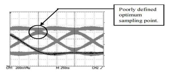
Figure 12-4. Distorted eye diagram
