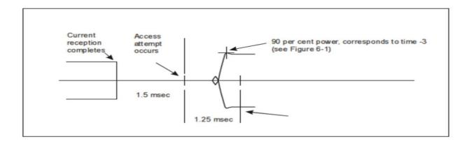
Figure 6-3. Receive to Transmit turnaround time
