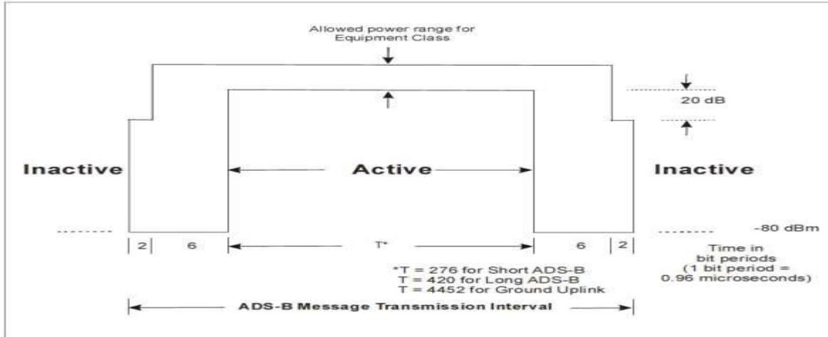
**Figure 12-2. Time/amplitude profile of UAT message transmission**
