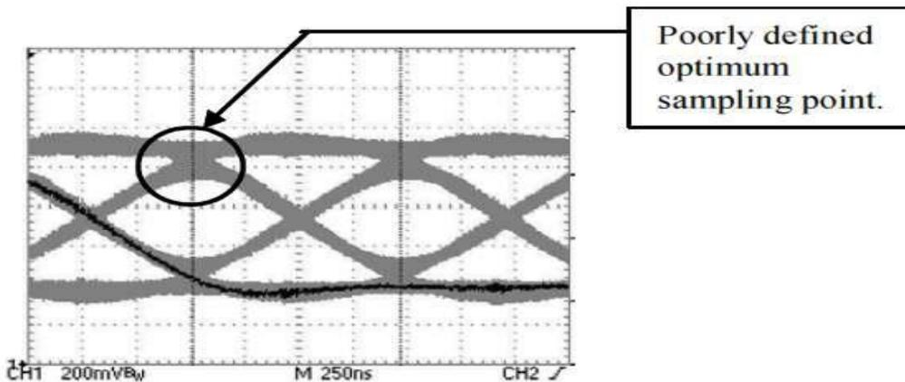
**Figure 12-4. Distorted eye diagram**
