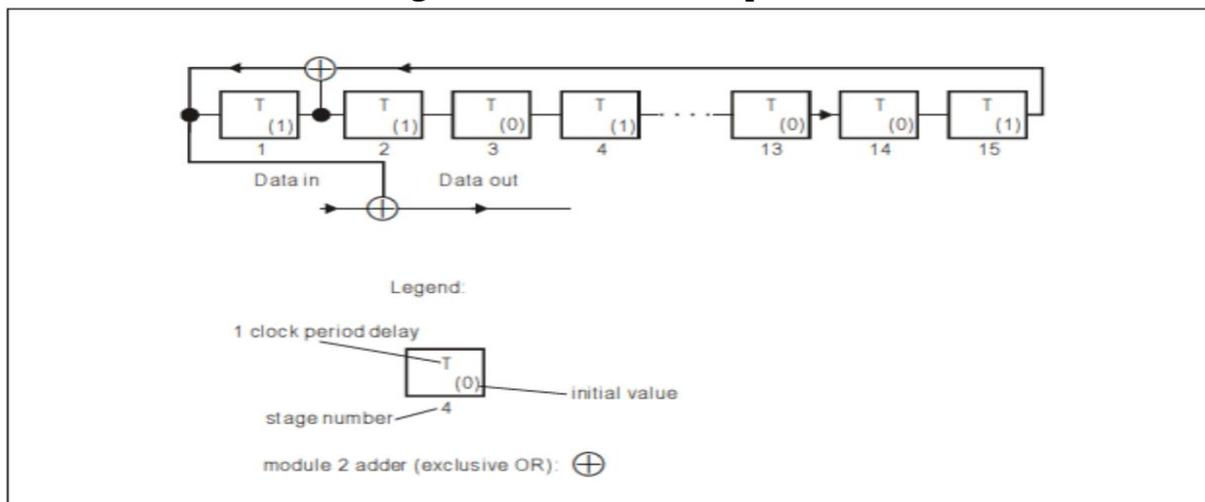
**Figure 6-2. PN-generator for bit scrambling sequence**
