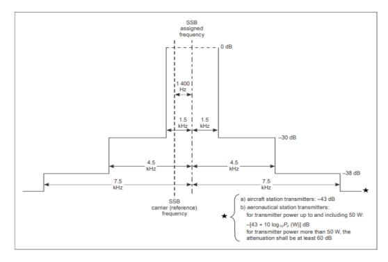
Figure 2-2. Required spectrum limits (in terms of peak power) for aircraft station transmitters first installed after 1 February 1983 and aeronautical station transmitters in use after 1 February 1983
