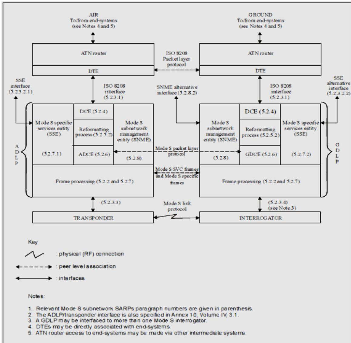
*Note. — Each Comm-A segment (MA field) received by the ADLP is accompanied by the first 32 bits of the interrogation that delivered the segment (23.4.3.1.2.10.5.2.1.1 of Subpart 4 of Part 23). Within these 32 bits is the 16-bit special designator (SD) field (23.4.3.1.2.6.1.4 of Subpart 4 of Part 23).*
