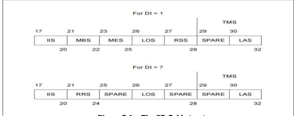
Figure 5-1. The SD field structure
