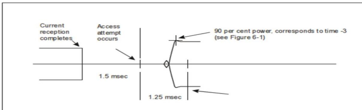
**Figure 6-3. Receive to Transmit turnaround time**
