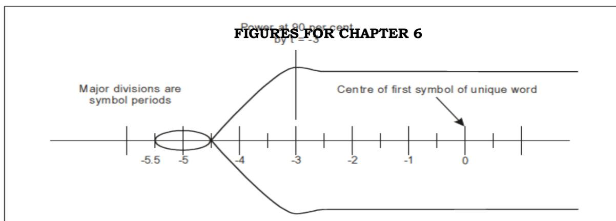
**Figure 6-1. Transmitter power stabilization**
