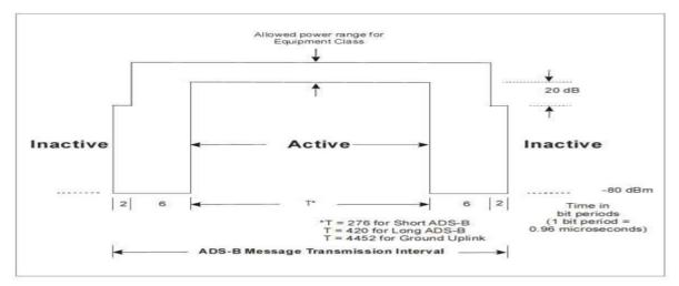
Figure 12-2. Time/amplitude profile of UAT message transmission
